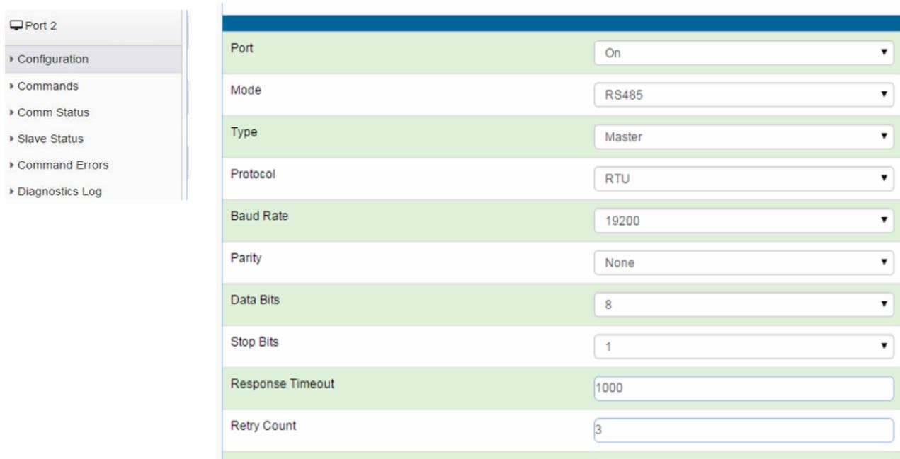
The screenshot shows the configuration interface for Modbus Port 2. The left sidebar lists navigation options: Port 2, Configuration (selected), Commands, Comm Status, Slave Status, Command Errors, and Diagnostics Log. The main panel displays the following configuration parameters:
