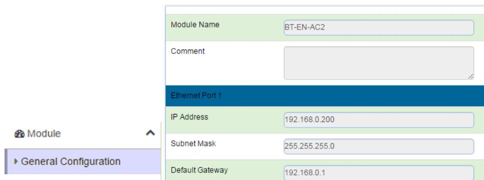
The screenshot shows the "General Configuration" page. The sidebar menu is partially visible with the "General Configuration" item selected. The main configuration area is for "Ethernet Port 1" and includes the following fields:
