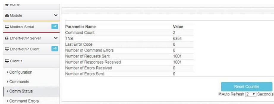
The screenshot shows the 'Comm Status' section of the Modbus Serial configuration. It displays the following data:
