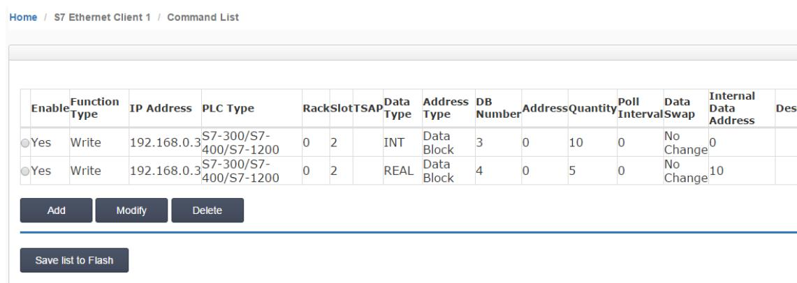
This screenshot shows the 'S7 Ethernet Client 1 / Command List' configuration interface. It features a table with the following columns: Enable, Function Type, IP Address, PLC Type, Rack, Slot, TSAP, Data Type, Address Type, DB Number, Address, Quantity, Poll Interval, Data Swap, Internal Data Address, and Desc. Two rows of data are present:
