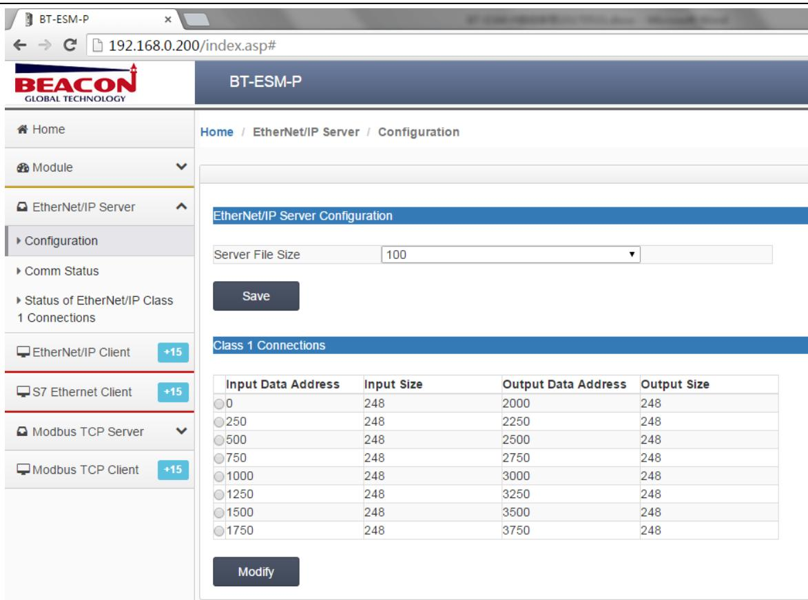
The screenshot shows the configuration interface for the BT-ESM-P module. The left sidebar lists various module types, with 'EtherNet/IP Client' and 'S7 Ethernet Client' currently selected. The main content area shows the 'EtherNet/IP Server Configuration' page, where the 'Server File Size' is set to 100. Below this is a table for 'Class 1 Connections' with the following data:
